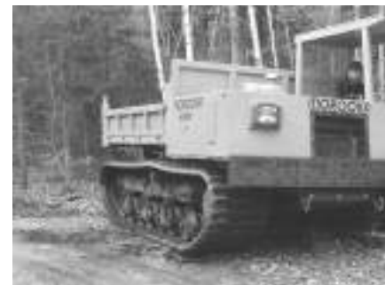
This Marooka will be used to transport construction materials deep into the woods with virtually no impact.
